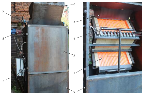
Electric furnace: 1 - case, 2 - unit (on the left picture the thermal covers are removed), 3 - door, 4 – dust collector, 5 - tray, 6 – drum dosing unit, 7 – thyristor regulator, 8 – dosing unit drive, 9 – belt drive,
